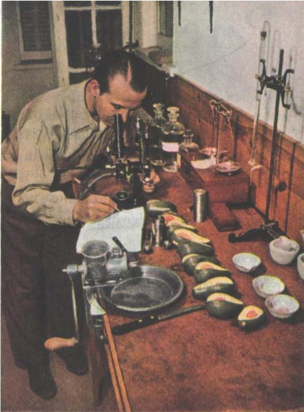
Oil content determines ripeness of the fruit. Chemists can give the answer after a series of laboratory tests.
